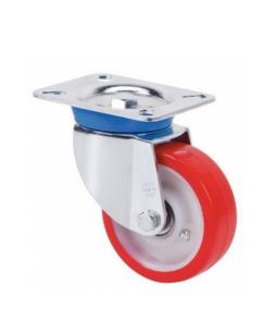
Castors with white nylon centre and red polyurethane tyre with a hardness of 90°-95° Shore A. Especially indicated to support high-loads up to 600kg (1323lb).
