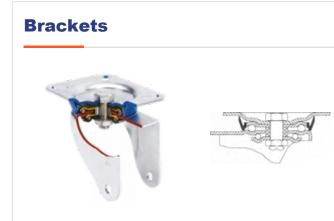
Manufactured with pressed steel up to 5 mm. Highly rustresistant double-chrome coating. Double ball bearing reinforced with hardened ball races. Dust-proof in the sealing swivel head. Manufactured to European standard EN 12532.
