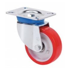
Castors with white nylon centre and red polyurethane tyre with a hardness of 90°-95° Shore A. Especially indicated to support high-loads up to 300kg (661lb).
