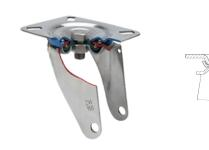
Made of high-quality pressed stainless steel (AISI 304) up to 3 mm. Bracket made completely of stainless steel, corrosion-free, resistant to petrol, diesel,oils and grease. Manufactured to European standards EN 12530/12532.
