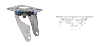
Made of high-quality pressed stainless steel (AISI 304) up to 3 mm. Bracket made completely of stainless steel, corrosion-free, resistant to petrol, diesel,oils and grease. Manufactured to European standards EN 12530/12532.
