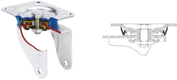
Manufactured with pressed steel up to 5 mm. Highly rust-resistant double-chrome coating. Double ball bearing reinforced with hardened ball races. Dust-proof in the sealing swivel head. Manufactured to European standard EN 12532.
