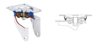
Manufactured with pressed steel up to 5 mm. Highly rustresistant double-chrome coating. Double ball bearing reinforced with hardened ball races. Dust-proof in the sealing swivel head. Manufactured to European standard EN 12532.
