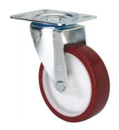
Castors with white polypropylene centre and brown cast polyurethane tyre with a hardness of 95° Shore A. Especially indicated to support high-loads up to 130kg (287lb).
