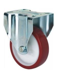
Castors with white polypropylene centre and brown cast polyurethane tyre with a hardness of 95° Shore A. Especially indicated to support high-loads up to 130kg (287lb).
