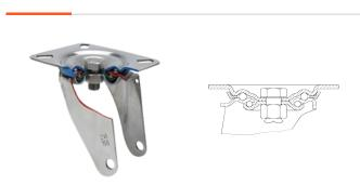
Made of high-quality pressed stainless steel (AISI 304) up to 3 mm. Bracket made completely of stainless steel, corrosion-free, resistant to petrol, diesel,oils and grease. Manufactured to European standards EN 12530/12532.
